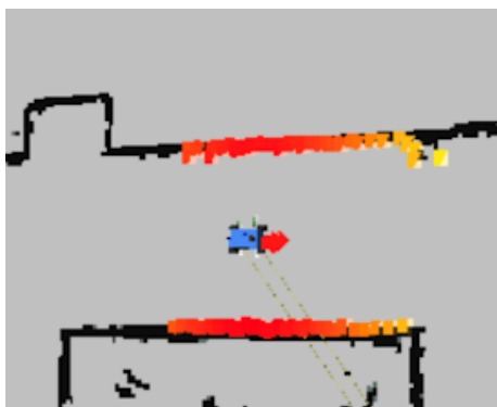
Figure 3: A cluster of 200 particles displaying the possible poses of the car after going through the sensor model and being resampled. Note that the large red mark in front of the car is actually 200 individual arrows representing the particles
